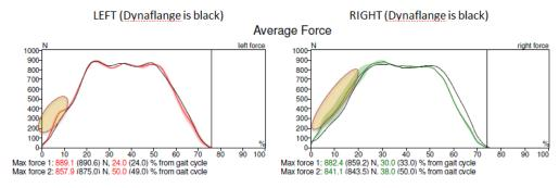
Figure 7 Left and right averaged GFR curves show reduced impact peaks at heel strike with DynaFlange<sup>™</sup>. There is also more steady loading which corresponds to increased control through mid-foot, leading to increased propulsion in DynaFlange<sup>™</sup> (Gray), versus "Legacy" (Red and Green).
